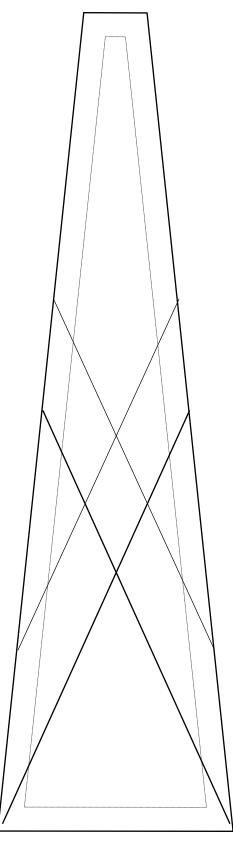
Trace the angled line onto the 12 degree wedge tool using a removable marker.
